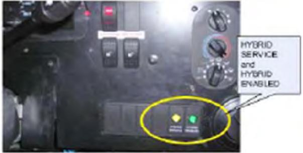
Further verification of the Hybrid Electric Vehicle can be made by:
