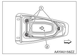
3. Remove the service plug using the following steps: (1) pull up and release the green lever, (2) press the locking tab to release and rotate fully upward, (3) pull the service plug completely out of its socket.
