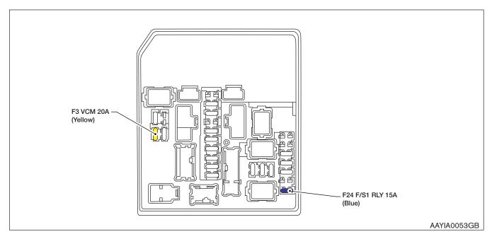
4. Remove the fuse box cover and remove the 20A VCM fuse.
