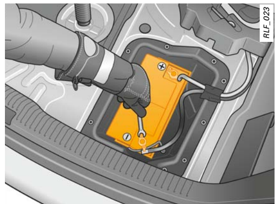
Illustration: Disconnection of the ground connection
