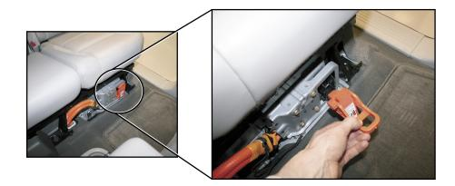
The service disconnect is located on the driver side front of the high voltage battery module. The plastic disconnect is colored bright orange. By removing this disconnect the high voltage battery circuit is interrupted.
