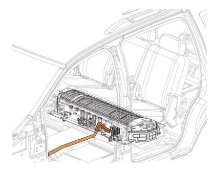
The DC high voltage cables originate at the high voltage battery. The connection is located on the driver side of the vehicle on the front of the battery.
