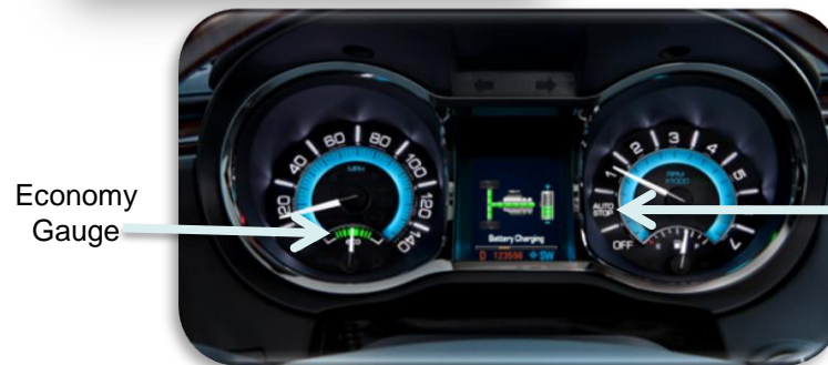
Auto Stop on Tachometer
