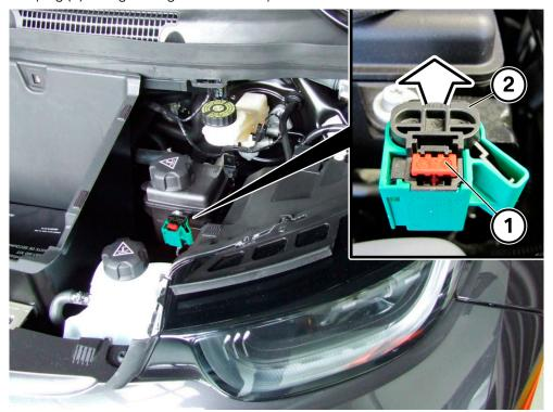
The high voltage system is deactivated when the hole (1) is clear all the way through.
