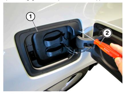
Cut through cable (1) for the high voltage disconnect (cutting solution). The high voltage system is deactivated.
