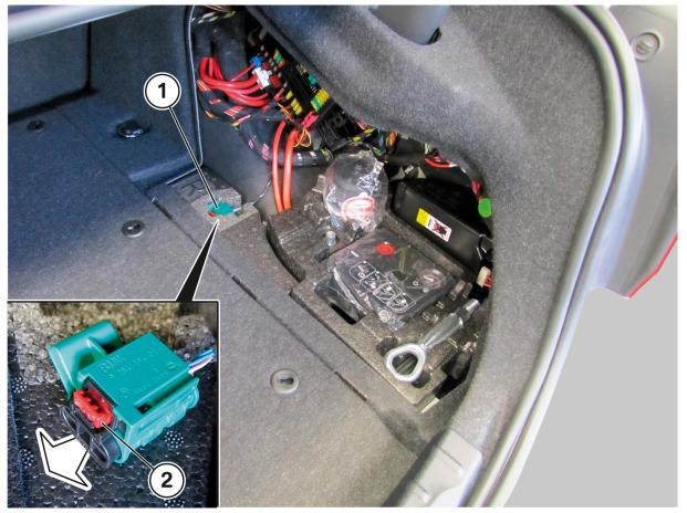
The high voltage system is deactivated when hole (1) is clear all the way through.
