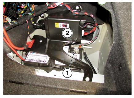
Disconnect the low voltage battery at the front:
