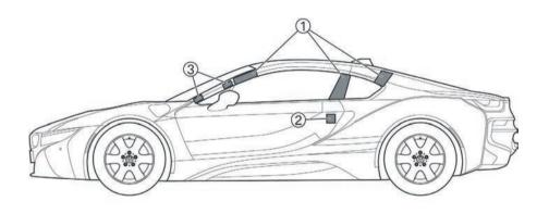
1 These areas indicate the points at which the roof can be severed. Modern high-performance cutters are required for cutting open the body; older hydraulic cutting devices may be insufficient.
