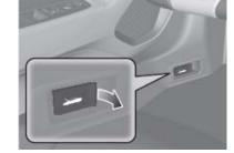
2. Locate the hood latch lever, push the lever, and lift the hood.
