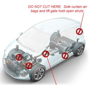
DO NOT CUT HERE. The Spark battery has 360 volt electrical potential at all times. It is located underneath the vehicle above the rear axle.
