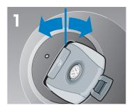
1. If the engine is running, turn the key to the left or to the right out of the neutral position, to turn off the engine. Remove the key if possible.
