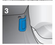
3. Find the access to the ground connection on the 12V battery. Move the driver seat all the way back, if possible.
