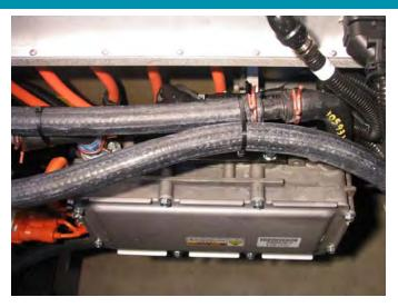
Orange cabling is found under the hood and underneath the vehicle to identify those wires carrying high voltage.
