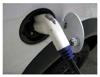
On the Right side of the vehicle – in the area normally occupied by the fuel cap – is the charge port.
