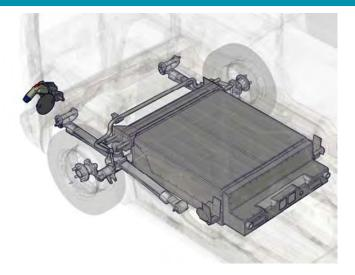
The sealed, liquid-cooled, high voltage battery pack is found under the vehicle – below the cargo area.
