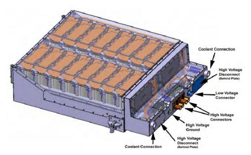
The high voltage battery pack consists of two strings of 8 battery modules in parallel.
