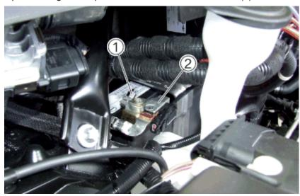
Slacken the nut (1) and pull off the battery earth lead (2) in the upwards direction.
