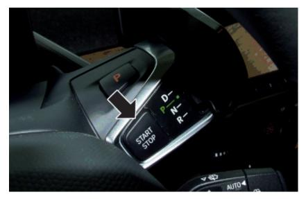
1. Press the START-STOP button, the system switches off.
