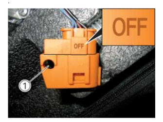
The high-voltage system is deactivated when bore hole (1) is completely free and the word "OFF" can be seen on the connector.
