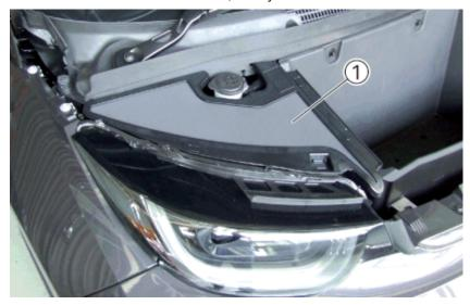
Open the engine compartment lid and remove the cover (1).
