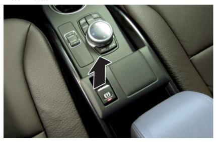
Pull the switch for the electrical Automatic Hold brake up.
