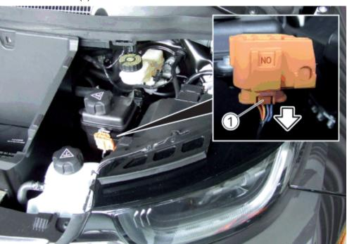
Unlock connector for high-voltage emergency separation point (1) and pull apart in direction of arrow.
