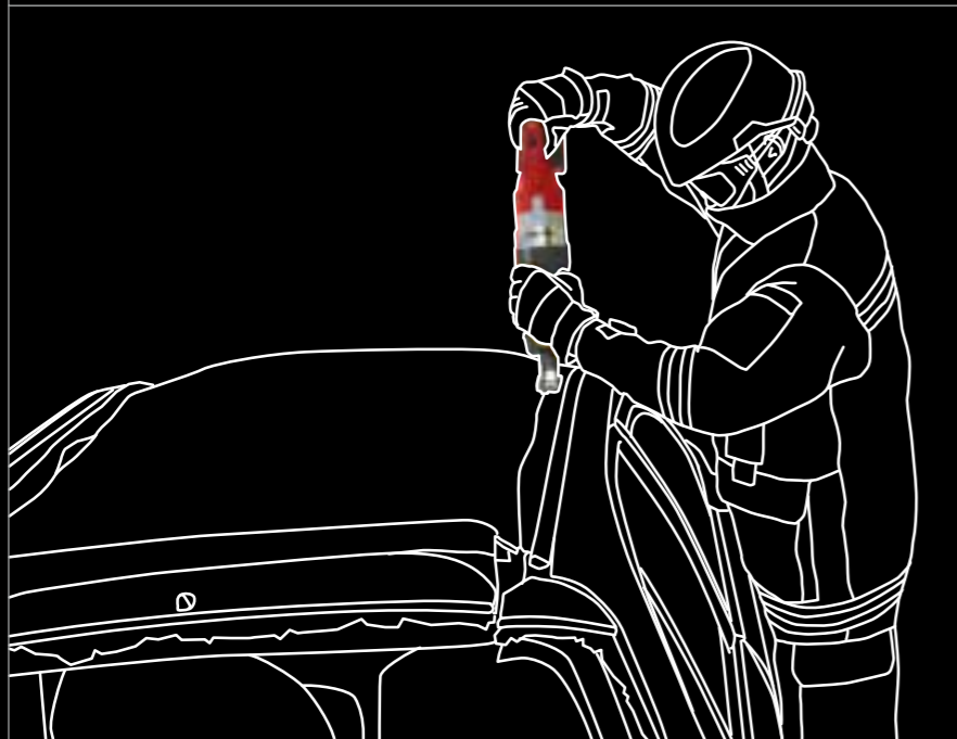
4 An rechter Dachreling entlang aufsagen Saw along right roof rack
