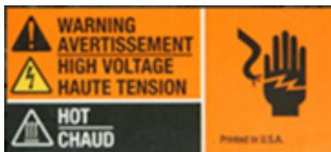
The high voltage warning labels are orange and indicate a potential shock hazard if high voltage is not properly disabled. The labels are located underneath the vehicle on all high voltage components, with the exception of the high voltage battery, which utilizes red danger labels. This tag will be visible if approaching a roll over incident.
