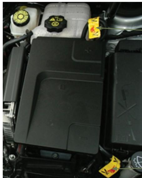
3. Cut auxiliary power module cable
