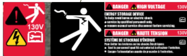
The high voltage danger labels are red and indicate that high voltage is present at all times. These labels are located on the high voltage battery in the trunk.
