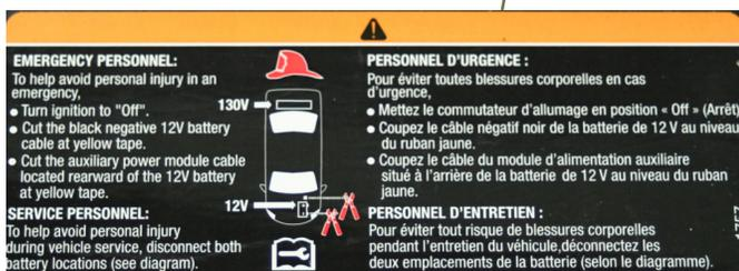
The first responder label located under the hood indicates the locations of the high voltage and low voltage batteries, as well as steps a first responder should take to disable the high voltage system.
