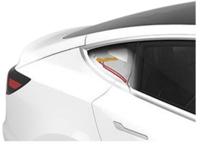
2. Use a reciprocating saw or hydraulic rescue cutters to cut 6 in (15 cm) through the rear pillar in the location shown.
