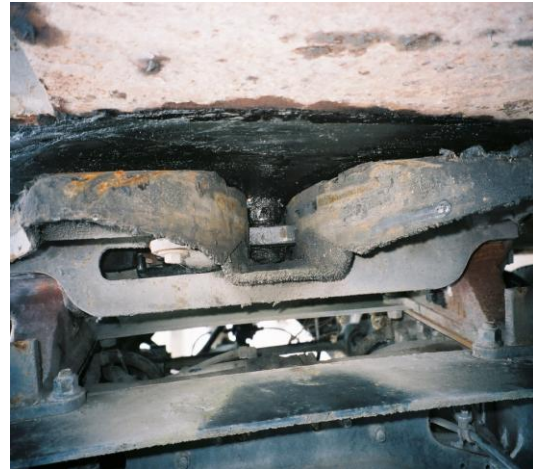
King Pin locked in place by drawbar
