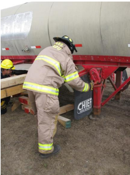
Lowering the landing gear by cranking
