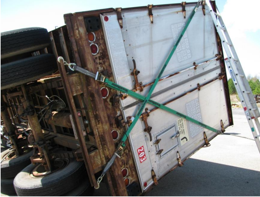
Cross strapping the rear of the trailer
