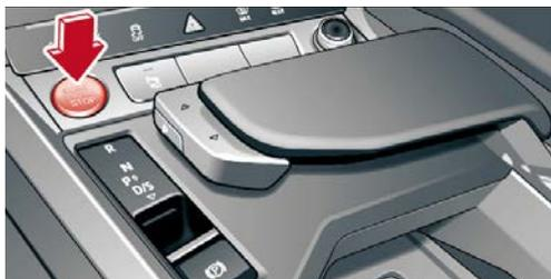
Press the START-STOP button without operating the brake pedal.
