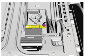
5. If equipped, position the battery cover insulator (1). Remove the battery disconnect access cover (2).
