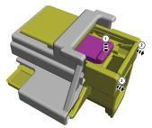
10. Insert a suitable tool inside the connector hole to prevent the connector from closing.
