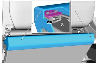
4. Position the LH front seat backrest cover and release a retainer (1). Position the LH front seat backrest cover (2).
