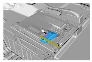
6. Remove the nut and position the battery cable. Torque 71 lb. in (8 Nm)
